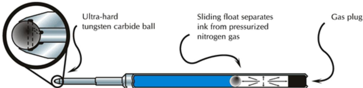
Stainless steel, precession-machined socket prevents leaks and oozing, yet delivers instant uniform ink flow
